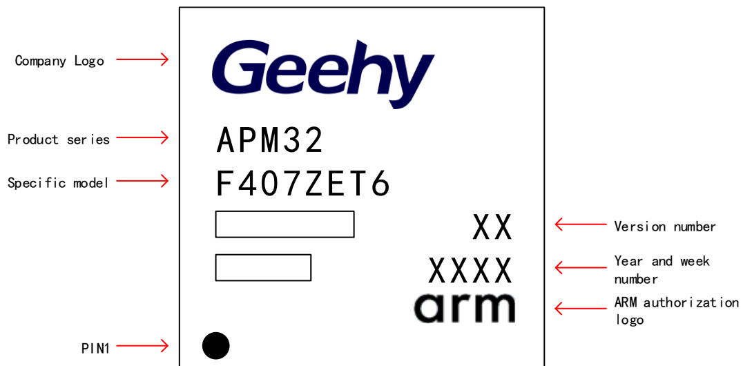
Figure 22 LQFP144 -144 Pins, 20 x20mm Schematic Diagram
